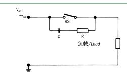
图2 Fig. 2 交流电感应性负载用RC连接法保护 Alternating current protection with RC link for inductive load.
